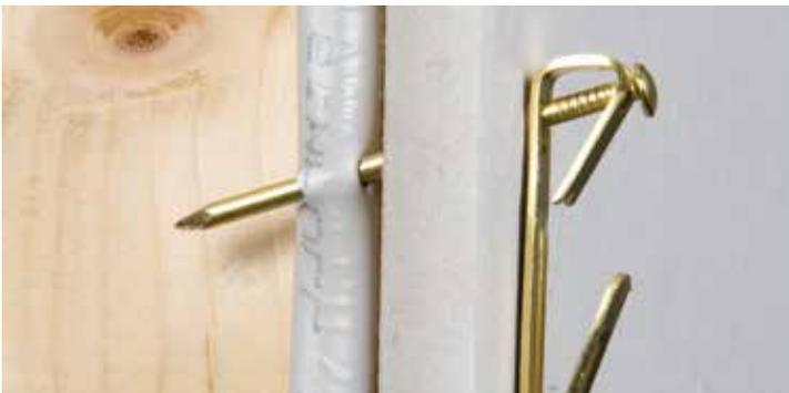
Photo 2: Example of line-to-ground arc fault (nail puncturing wire).
