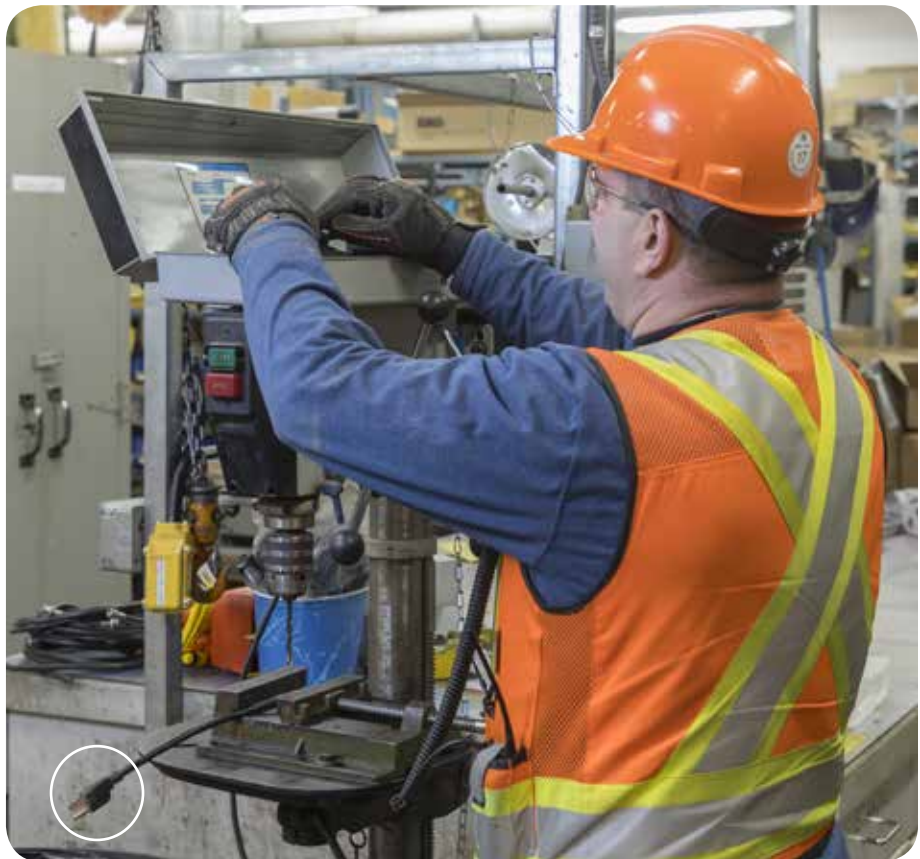
Figure 17: A worker servicing plugged-in equipment. The plug is under his exclusive and immediate control (placed in front of him, with his body as a barrier).
