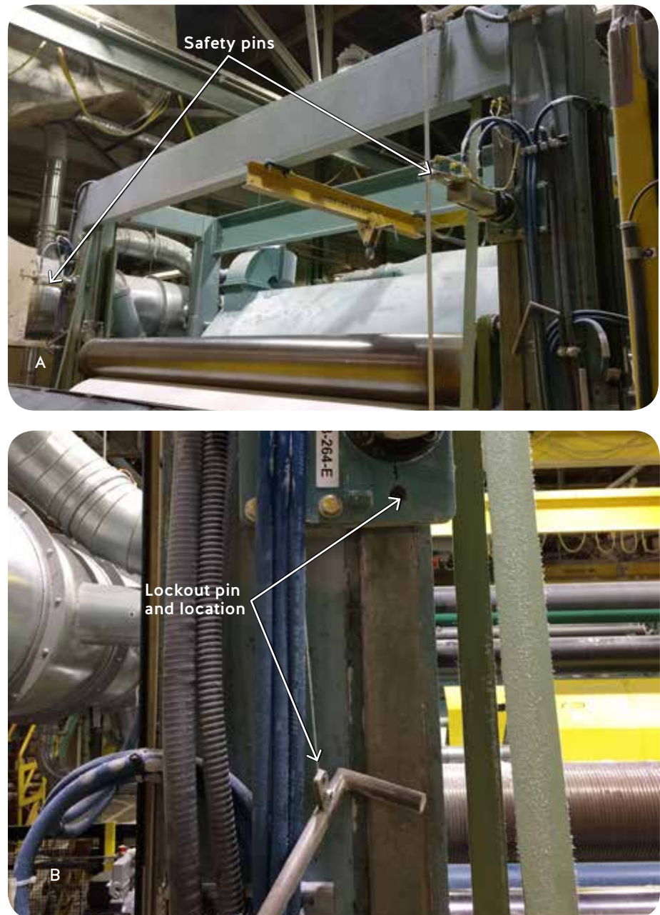
Figure 19: Pins used for safeguarding and lockout. (A) Safety pins that are part of a machine's safeguarding system for normal operating activities. (B) Lockout pin to be used during maintenance.
