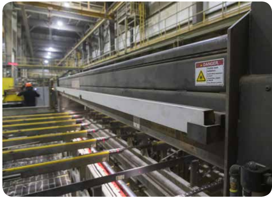
Figure 1: An example of radiation energy in industry: a laser system installed on a lumber trimmer.
